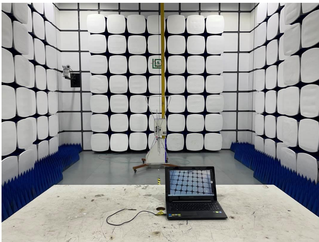
Test Setup Photo of Radiated Measurement (30MHz~1GHz)
