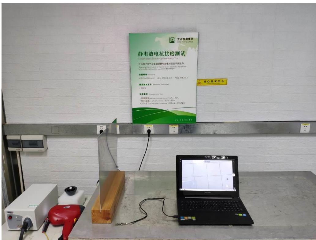
Test Setup Photo of Electrostatic Discharge Test
